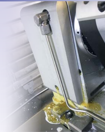
severe oil loss
