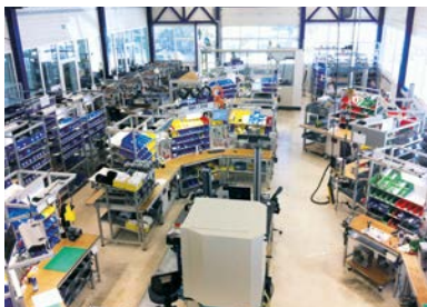
Assembly area with Kanban System
