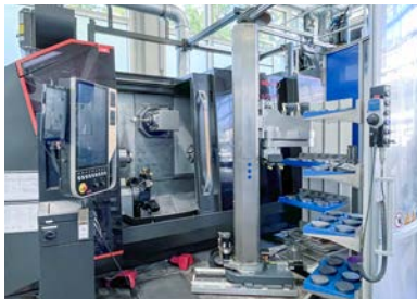
With workpiece pool for unmanned production
