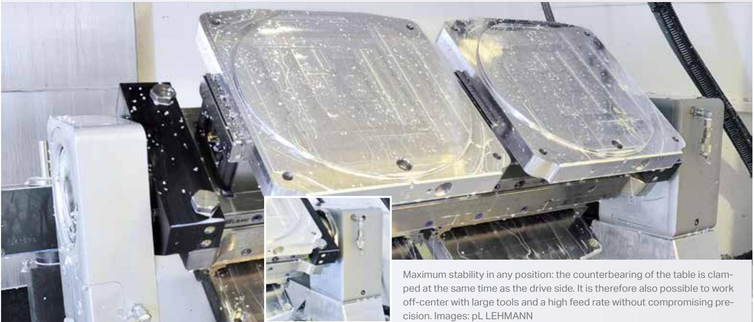
Maximum stability in any position: the counterbearing of the table is clamped at the same time as the drive side. It is therefore also possible to work off-center with large tools and a high feed rate without compromising precision. Images: pL LEHMANN
