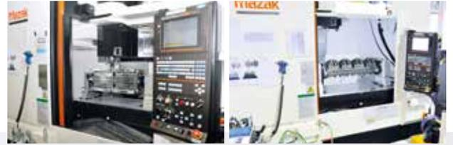
3+1 axes – a successful combination: At SMC, the Mazak machining centers equipped with pL LEHMANN rotary tables achieve a significant efficiency increase and high precision. Images: pL LEHMANN
