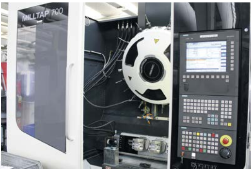
3+2 axes - a successful combination: At WSS, the DMG MORI Milltap 700 machines equipped with pL Lehmann rotary tables achieve a significant efficiency increase and high precision.
