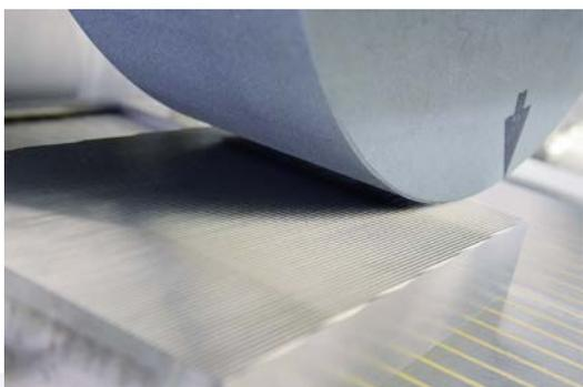
Grinding a thread-rolling die with inlet and outlet tapers.
