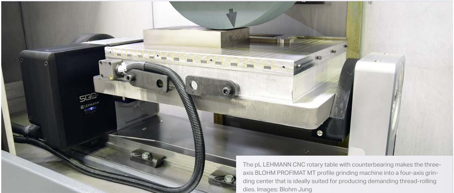
The pL LEHMANN CNC rotary table with counterbearing makes the three-axis BLOHM PROFIMAT MT profile grinding machine into a four-axis grinding center that is ideally suited for producing demanding thread-rolling dies. Images: Blohm Jung
