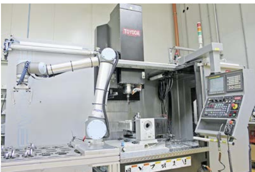
The Toyota FV1165 machining center was automated with a URC articulated-arm robot by MBN. Result: 20 percent greater productivity.
