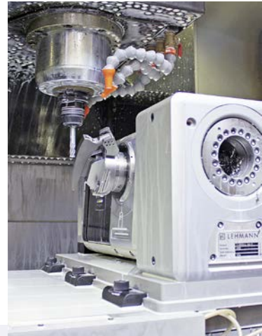
The pL LEHMANN T1-510520.LL fixX CNC rotary table converts the vertical, three-axis Toyota milling machine into a five-axis machining center for complete machining of complex parts.
