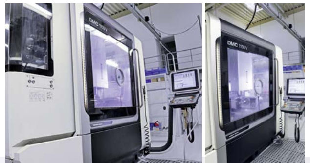
In 2015, Jongen added two DMG MORI DMC 1150V machines, which together with the additional T1-520520.RR varioX tilting rotary table from pL LEHMANN can machine in five axes.
