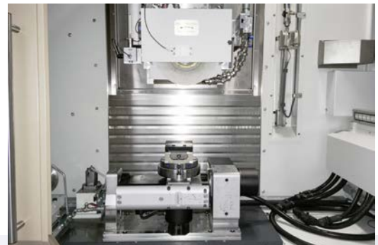
Used grinding wheel with 300 mm diameter, including two dressing points. The rear part for flat dressing and back-dressing of the grinding wheel, at the front a forming roller for profile dressing.
