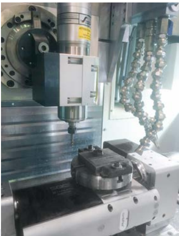
The clamped milling cutter is used for surface finishing of the layers applied by LMD.
