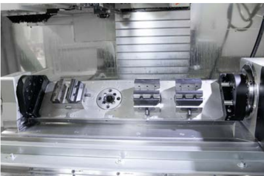
The different equipment of the rotoFIX clamping yoke from pL LEHMANN using three Gressel C2 125 centric clamps in this case; thus short or long workpieces can be clamped and completely machined with 4 axes.
