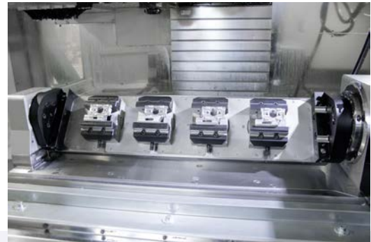
Complete equipment of the clamping yoke with, in this case, four Gressel C2 125 centric clamps for successive 4-axis machining of identical or different workpieces.
