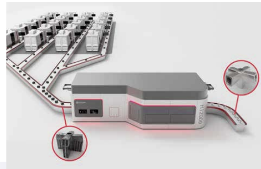
at left: The process can also be set up for incoming large quantities in finishing lines using an H12000 with a capacity of 500 parts per hour. at right: The stainless steel vacuum gripper is freed from the supports and ready for use after finishing by means of Hirtisation®. (Images: Materialise)
