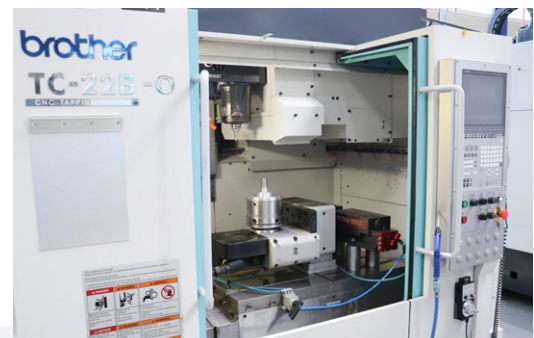
An optimal manufacturing solution, especially for job shops: a three-axis milling machine with an additional two-axis CNC rotary table from pL LEHMANN, which gives the machines five-axis capabilities.
