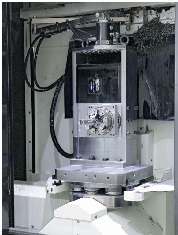
pL CNC axes can also be employed usefully on horizontal machining centers. Thus, the original four-axis machining center becomes a 5-axis center.
