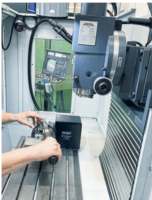
The originally 3-axis Avia machine is equipped with an EA-510-M3 rotary table from Peter Lehmann. This enables 4-axis simultaneous machining with Hypermill programming.
