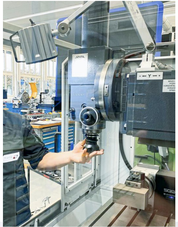
The new Avia machine is equipped with a hydraulically operated tool unclamping system for SK40 69871 A tool holders.
