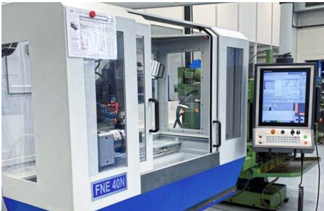
The manually and CNC operated Avia FNE40 N tool milling machine is equipped with an up-to-date Heidenhain TNC620 HSCI control system.
