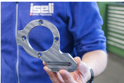
ISELI manufactures the components needed for its machines in-house. This sample component was completely machined on the automated Makino PS105 with pL rotary table.
