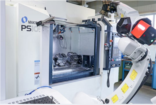
High productivity in a small space – the 3+1-axis production cell installed at Iseli is easy to set up and impresses with process-reliable automatic operation.
