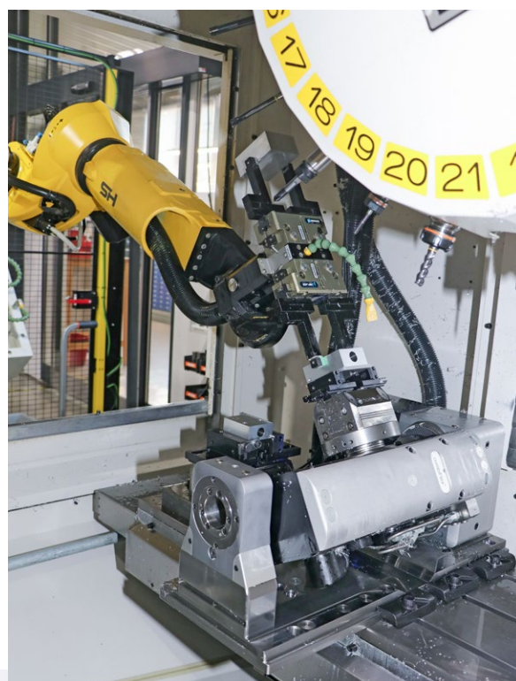
With its dual gripper, the robot loads and unloads the clamping device on the pL rotary table. It also performs alignment, measuring and cleaning tasks.
